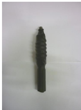
Loading coil assembly after encapsulation with heatshrink. The top thread just visible is 24TPI 5/16" (commonly called "Australian thread" as commonly used on CB and some amateur & land mobile antennas). Inside the bottom metal section is again the same 5/16" thread.
