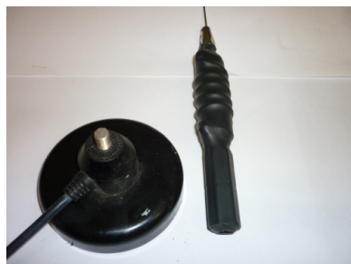
Loading coil assembly after encapsulation with heatshrink. The top thread just visible is 24TPI 5/16" (commonly called "Australian thread" as commonly used on CB and some amateur & land mobile antennas). Inside the bottom metal section is again the same 5/16" thread.
